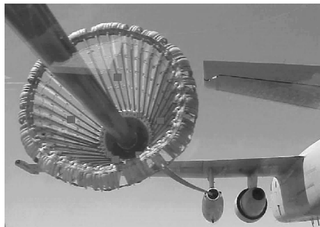
Fig. 4 Conceptual VisNav LED beacon configuration on drogue basket.
